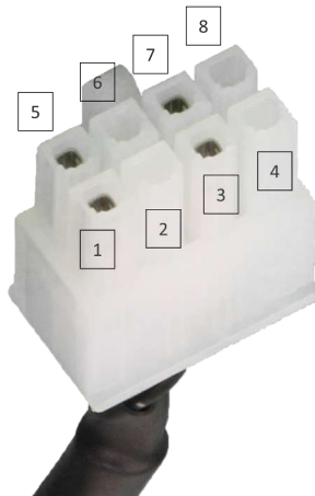
Fig. 3: Molex connector PIN assignment
