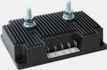
The CDR can be installed between the starter and auxiliary battery as an electronic battery isolator. The device can be used both bi-directionally and unidirectionally. The batteries are charged almost loss-free and the plastic housing protects against short circuits. Thanks to a switch-off function, it can also be used as a main switch to connect/disconnect a consumer or an on-board network.
